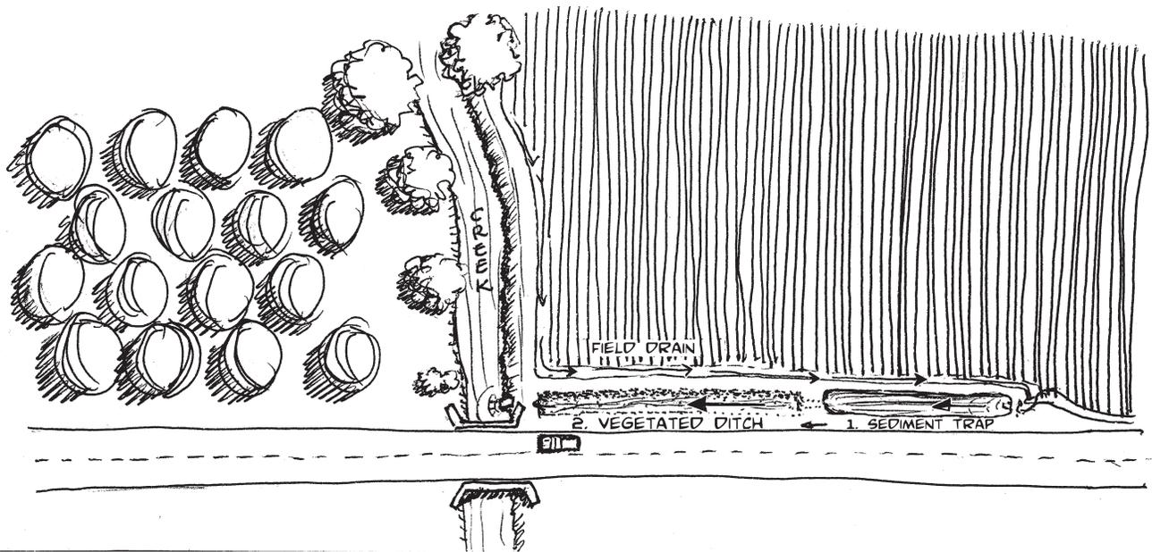
In this field, furrows drain from top to bottom of the picture. Water is captured in the tail ditch and passes through an up-stream sediment trap from right to left before entering the vegetated ditch enroute to the stream (see arrows).
